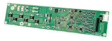
▶ Battery Management System
